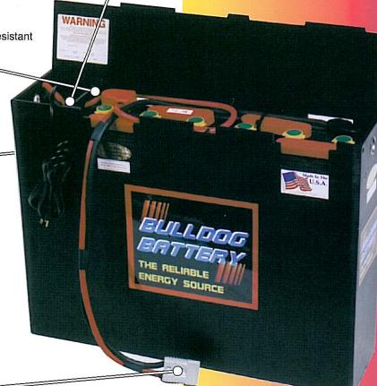
The battery and charger are connected with an SB connector. An additional set of leads are provided for the truck connection. All that is required to charge this battery is a 120 volt AC wall outlet. The operator does not need to unplug the battery from the truck and then plug the charger into the battery. This system will eliminate the error of charging with truck instead of the battery.
